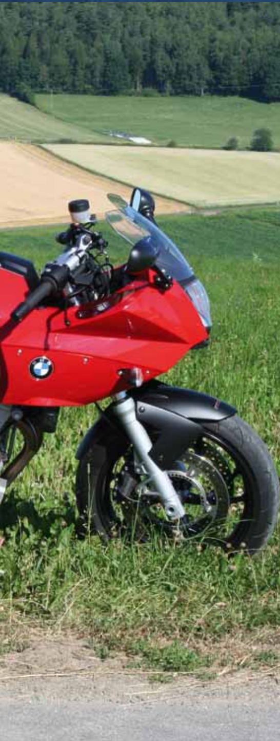
Windshield V-Stream, design flat, clear, with homologation, Height 42 cm, Width 41 cm
