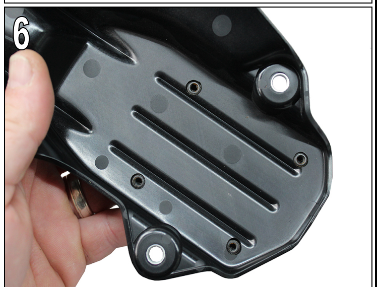
Fig. 6 Place AC Schnitzer cover on standard starter motor cover. Bars of the AC Schnitzer cover must be aligned with the holes.
