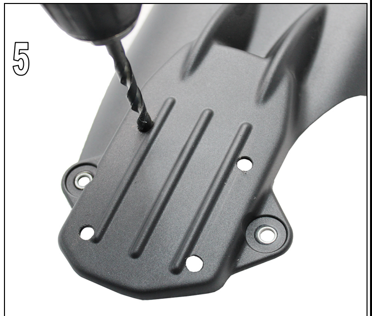
Fig. 5 Drill out the transferred markings carefully and in the centre using a \varnothing 6.5 mm drill bit
