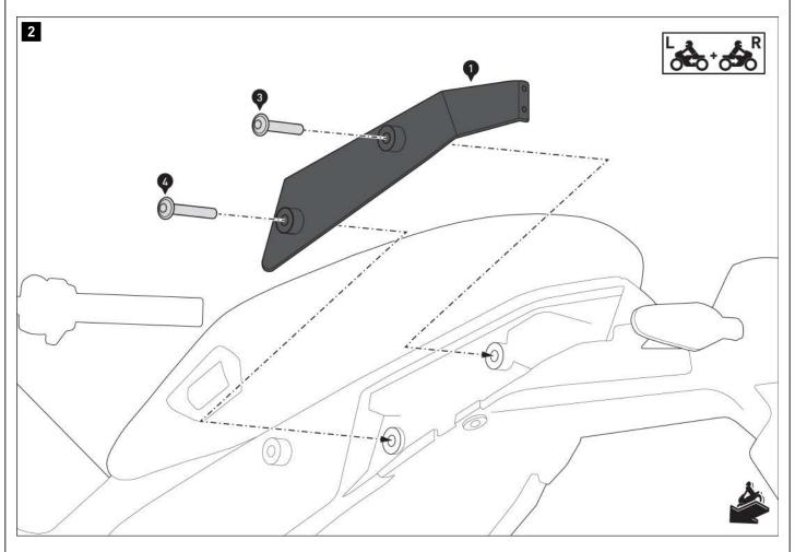
Mount the cover plates (1) and (2) on both sides of the vehicle. **A WARNING: Use a liquid threadlocker!**Do not tighten the screws (3) and (4) yet.
