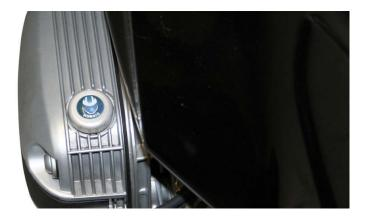
There is a drilling in the side of the plug in which you can put a size 3 Allen key or a Torx key T10 (usually found in your BMW toolkit) in order to fit and remove it. See tools.
