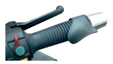
Our throttle control is a device that easily wraps around the throttle grip of any motorcycle. It protrudes away from the grip so that the contoured portion fits comfortably against the heel and palm of the hand. Using the heel of his hand, the rider applies minimal downward pressure onto the throttle control, making the throttle rotate. Additionally, the throttle control works as a resting place for the hand, reducing fatigue on long trips.
