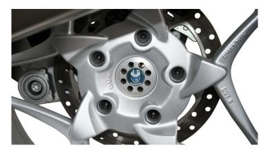
Rear wheel centre cover with emblem. The holes in the covers aid cooling! Measured temperature on the engine test stand (engine is cooled with a supercharger) without plug: 54,9C; with plug: 50,1C Measured temperature after a tour of about 250km without plug: 53,4C; with plug: 49,4C.
