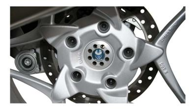
Rear wheel centre cover with emblem. The holes in the covers aid cooling! Measured temperature on the engine test stand (engine is cooled with a supercharger) without plug: 54,9C; with plug: 50,1C Measured temperature after a tour of about 250km without plug: 53,4C; with plug: 49,4C.
