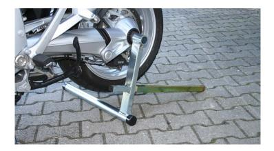
Slide the rubber coated pipe of the back lifter into the final drive of your BMW and lift it up. Easy to use by one person and very stable support for the bike.
