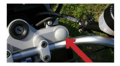
Nice looking cover for the fork tube which works as a replacement for all plastic caps, kept firmly in place by an o-ring. In order to replace all plastic caps you get 2 covers in a set.
