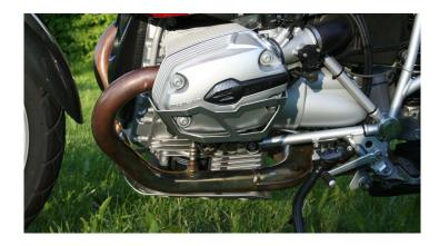
Made of 3 mm aluminium with the latest laser-cutting and bending technology. Available in 2 versions (with/without grid) with 2 colours (natural/black anodized). Images 1 - 4. Easy and fast mounting to the original attachment points. 1 set (for left & right side) incl. fasteners and install instructions.
