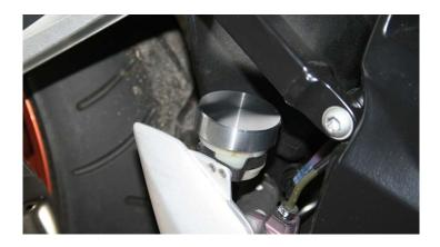
Cover for the foot brake fluid reservoir, CNC machined of aluminium. Image shows K1200R, but it is also visible on: K1200RS without Int. ABS K1200S R1200S, R, ST & GS R850, 1100, 1150GS & R850, 1100R. If you do not have any silicone at home, you can also order our high-quality silicone which is pre-filled in the volume you need and easy to dose.
