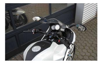
These handlebars create a new sporty looking and improve the handling of your bike. The mounting kit is made of high quality aluminium and the bars are especially designed for the BMW K1300R. Width of the handlebar is ca. 770mm.
