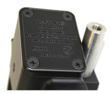
Our mirror heightenings are the perfect solution if you mainly see your shoulders in the rear mirrors. The mirrors will be placed 3,0 centimeters higher and that creates the necessary space in order to improve the view to the back.
