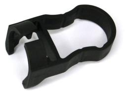
The spark plug connector of the new generation bikes makes it easy and secure to remove the spark plug connector. The connector is actually the coil as well. This tool makes it easy to remove the spark plug connector / high tension coil. Attempting to remove the connector without the proper tool will not only be difficult, it may cause irreparable damage to the connector.
