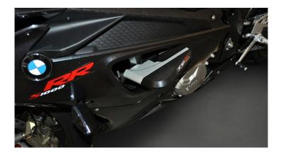
Our Crash-Protectors or Sliders protect your frame, engine and fairing of your motorcycle. This crash protector is designed to fit perfet to your motorcycle. It is made of high-strength milled aluminum and high-strength POM plastic. All our pads are screwed to your motorcyle at least at 2-3 points. The advantage over round crash protectors is that these slider can't break or snag on something on the road.
