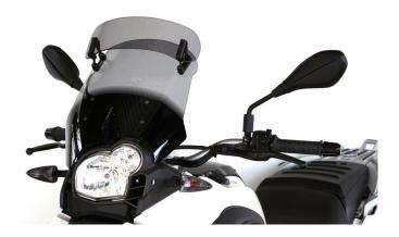
This Vario touring windshield for BMW G650GS & G650GS Sertao has a spoiler at the top of the airfoil; the spoiler can be adjusted for height and angle in seven positions. The air current deflected behind the spoiler reduces the otherwise annoying turbulence.
