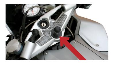
This GPS Mounting for BMW K1200 and K1300 motorcycles will be mounted to the upper fork crown instead of the BMW emblem. This black GPS Mount has a 1 inch RAM ball where you can mount almost any GPS unit for example with our clamps. Diameter RAM ball: 1 inch (2,54 cm)
