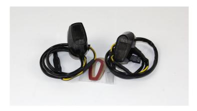
You simple glue these LED Fairing Turning Signals in the turning signal space in front of the S1000R's fairing with a 3M foil. The indicators have an e-mark and are road legal.
