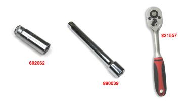
You will need a special small and long wrench socket size 14mm to remove the spark plugs of your BMW LC engine (article number 682062). In addition to the wrench socket you will need an extension (article number 880039) and the correct 3/8inch ratchet wrench (article number 821557).
