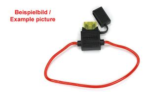
This fuse holder includes a 20A flat fuse and can be added to a plus-cable of a electric device, for example additional lights, GPS units or horns. You can use fuses from 1A - 30A.
