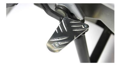
This special part is made of an extremly handy aluminium and cares for safe braking. It gets mounted with two screws, u-screws, nut and hulls which are all yet with the enlargement.
