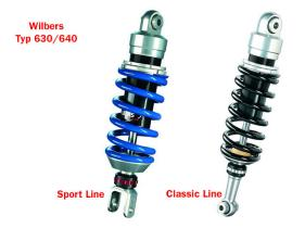
The basic Wilbers Racing Suspension shock absorber is adjustable in rebound and preload. Depending on the article number it is either the shock 630 with 36 mm diameter or the version 640 with 46 mm diameter. With many motorcycle models the shocks can be assembled individually to raise or lower the seating height. Wilbers Suspension rear without external compensating reservoir.
