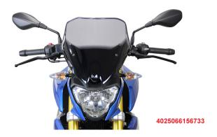
Our Naked Bike Racing Screen for BMW G310R motorcycles fits perfectly to this agile, easy-to-use and lightweight Roadster. At a height of 32 cm and a width of 32 cm, the screen shields from headwind while highlighting the ease of use and the strengths of this city runabout. The windshield mounts onto two angle brackets on the handlebar clamp (mounting hardware kit included).
