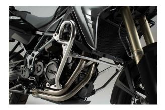
Our crash bars are made of high-quality stainless steel and are especially designed for your F650/700/800GS. The crash bars are designed to be very robust and allow for an equal distribution of forces in a crash. You and your bike are protected in the best possible way. Crash bars offer a very good protection, but they can reduce the cornering angle.
