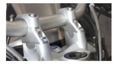
Handlebar risers with offset: 30mm higher and 21mm closer to the rider
