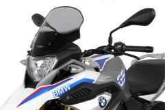
The touring shield has the same shape as the original windshield, but with an additional raised wind deflector at the top, covering the entire width. This deflects the wind over the rider and allows a relaxed ride, particularly on longer trips.
