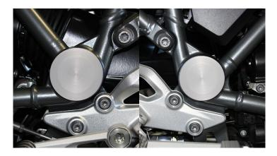
These aluminium parts cover the big holes above the foot pegs of your BMW and make sure that no dirt or dust can stay in it, water can still escape.
