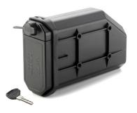
This toolbox, which will be mounted between the side case mounting PLR5108 or PL5108CAM and the motorcycle, is made from techno-polymer, is waterproof and has a internal removable partition. The toolbox has a Security Lock with dust cover which can be mounted in both directions, so that the lock is either on top or at the bottom.
