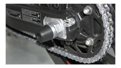
These crash protectors for the rear swingarm are made of cnc lathed plastic (POM). The mounting is made of cnc milled and anodized aluminum.
