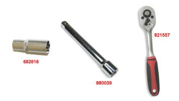
You will need a special small and long wrench socket size 16mm to remove the spark plugs of your BMW engine (article number 682016). In addition to the wrench socket you will need an extension (article number 880039) and the correct 3/8inch ratchet wrench (article number 821557).
