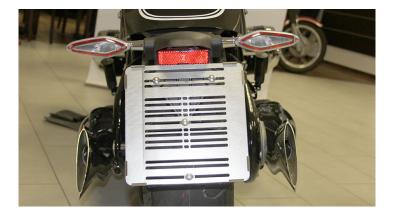
This adjustable licence plate bracket is made of high-quality stainless steel. You can adjust the width from 18 to 28 cm. The height of the licence plate is 20,3 cm.
