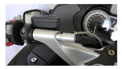
With this adapter, items that have a 22mm tubular handlebar clamp can be securely attached to the motorcycle. The adapter is screwed to the handlebars from the inside.
