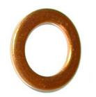
Washer for fork tube drain plug. The ring has an inner diameter of 8mm, an outer diameter of 12mm and a thickness of 1,5mm.
