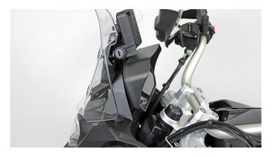
Sun visor for 6.5 inch display, suitable for the Connectivity instrument cluster. With this high-quality glare protection, the display remains easy to read even when the sun is low. Made from UV-resistant and durable plastic, it offers very good protection against direct sunlight. Very easy to install - just plug it in and it clicks into place.
