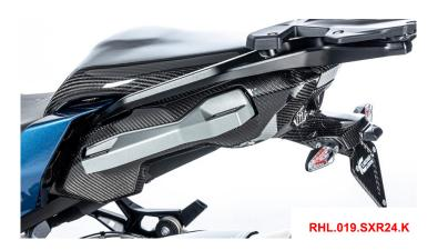
The Carbon Fiber rear subframe cover for the tail of your BMW S1000XR (2024- ) consists of two parts which get fixed on the left and right sides of the bike. Made of high quality carbon fibre.
