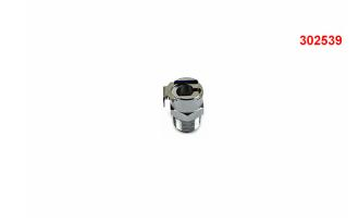
If the quick coupling on the fuel pump becomes leaky, the entire pump does not need to be replaced. You can replace the quick coupling with our repair kit. Like the original, the quick coupling is provided with a thread and a shut-off valve and has a fuel-resistant Viton seal.
