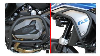
These crash bars are made of high-quality steel (black powder-coated, satin-finished) specifically for the BMW R1300GS and perfectly match the look of the motorcycle and the shape and the colour of the boxer engine. The crash bar is very stable and ensures an even distribution of forces, which means you and your motorcycle are optimally protected. The crash bar does not have to be removed for standard customer service work and is mounted on the original screw points.
