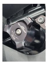
This adjuster for the rear shock absorber impresses with its first-class feel and high-quality workmanship. Instead of the standard plastic component, it is made of precisely machined, black anodized aluminum. This not only ensures comfortable and safe handling but also gives the component a sophisticated, vehicle-specific appearance. A perfect upgrade for drivers who value functionality and design at the highest level.
